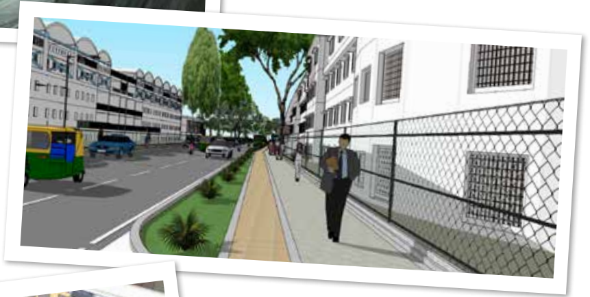
Redesign of Vittal Mallya Road as per Tender S.U.R.E. guidelines, with uniform travel lane widths, continuous footpaths, a designated cycle track and landscape strips.
